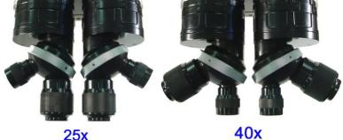
eyepieces are 40x magnification, the larger ones are 25x magnification. Rotate the turrets until they snap into position, as shown below. It's best to start with the 25x eyepieces.
