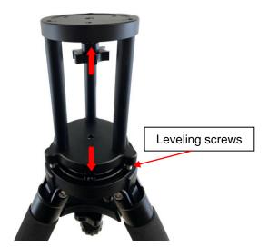
(5) Adjust the leveling screws with a screw driver or a Allen wrench;
