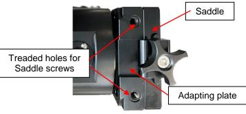
Remove dovetail saddle from the adapting plate by unscrew four socket screws;
