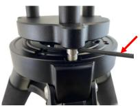
(6) Fully tighten both tripod center bolt and tripod tray locking knob while monitoring the level.
