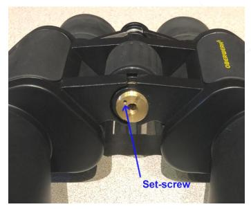
To remove the brass tripod adapter socket, loosen the small set-screw (as shown above), then unscrew the socket using a large flat-blade screwdriver. Install the mount adapter in its place, then tighten the set-screw to prevent the adapter from loosening.
