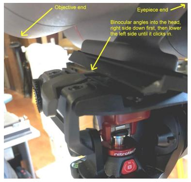
balance. Safety stops will prevent the binocular from traveling too far in each direction. Once balanced, move the lever forward to lock the Q/R plate.
