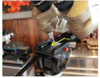
Focus one eye at a time by turning the large knurled focus rings in between the prism housings and the eyepieces.
